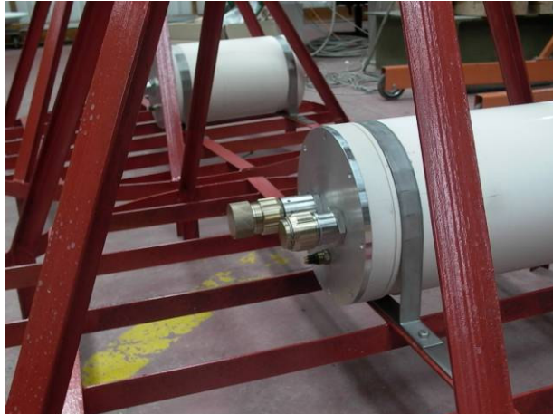
Underwater nodes and metallic structure for quick deployment
