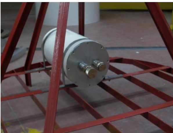
Underwater nodes and metallic structure for quick deployment
